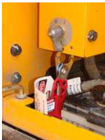
Positive Isolation Point on Excavator
