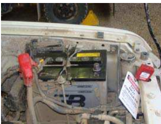
Disconnect and lock out earth lead off light vehicle battery.
